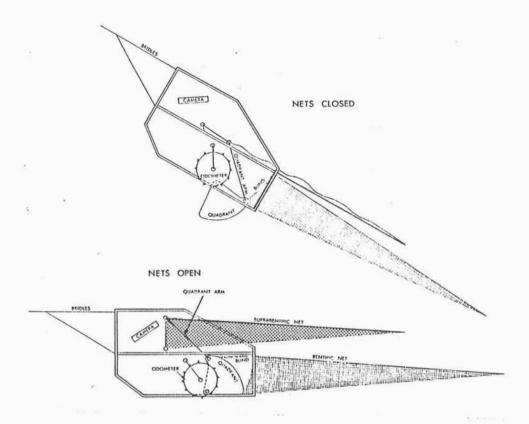
The increased height of the frame has allowed the camera to be raised and consequently set at a steeper angle. The smaller area photographed is more than compensated for by the less oblique angle and subsequent increase in detail, making quantitative analysis easier and more accurate.
